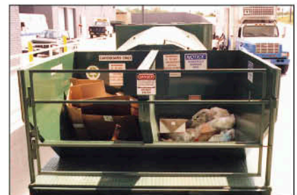
At this large hospital, the DRC II averages 60% trash in one compartment and 40% cardboard in the other compartment. This provides convenience and flexibility with only one unit.
