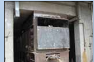
This M-1475XW Transfer Station Compactor is fed via a tipping floor and features the Scissor trailer connection system.
